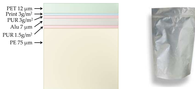
Figure 29: standard aluminium laminated plastic pouch
